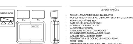
LUMINÁRIA DE EMERGÊNCIA - TIPO REFLETOR SEM ESCALA
