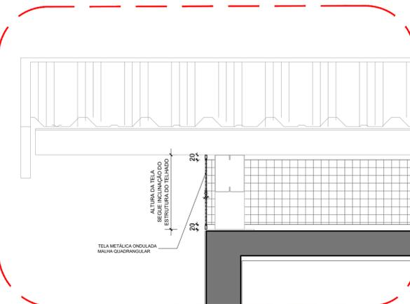
**DETALHE - TELA METÁLICA CORTE ESC. 1/10**
